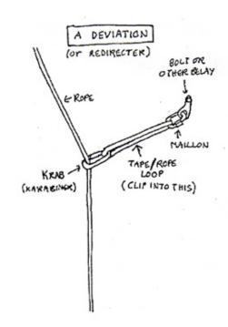
A deviation (or redirector) is another means of avoiding rub points and other hazards by altering the hang of the rope down the pitch. The rope runs freely through a krab which is attached to a belay via a tape or rope-loop. This deviation pulls the rope away slightly from its natural vertical hang to move the rope below the deviation away from a rub-point. A deviation never bears the full weight of a caver (or a fraction of it) and consequently
